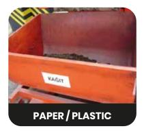
Since the paper and plastic from the process are contaminated with oil, their calorific value is between 5000 - 6000 kcal/kg. This product is valuable fuel for cement factories
